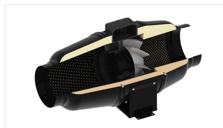
Due to the conic impeller and special blade profiling the circumferential air speed increases thus providing higher air pressure and capacity as compared to standard axial fans. The diffuser, the specially profiled impeller and the directing vanes at outlet from the fan casing distribute air flow in such a way as to attain the best combination of high performance and high pressure at low noise level. The fan casing is equipped with an airtight terminal box for connection to power mains.
